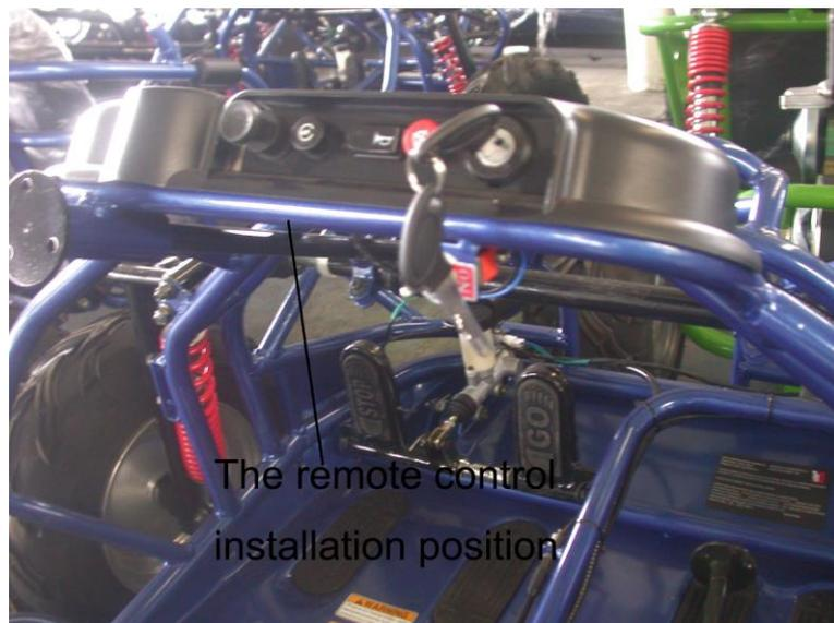
3. The purpose of this remote: remote control to shut down the engine. Guardians could use this remote to shut down the engine in the emergency to avoid accidents.
