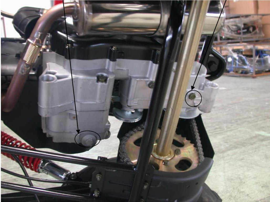
2. 150cc Engine transmission case oil lube plug, crankcase oil lube plug:
