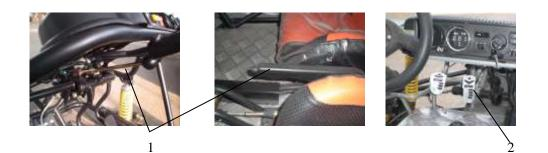
1.Parking brake plate 2.Throttle lever
