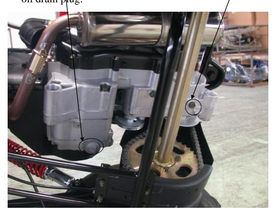
2. 150cc Engine transmission case oil lube plug, crankcase oil lube plug:
